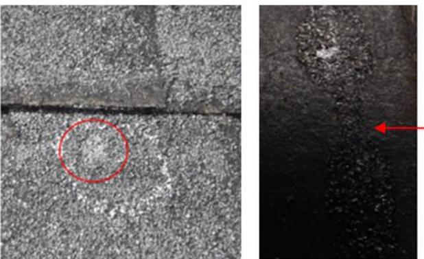
Pass - No Cracking
